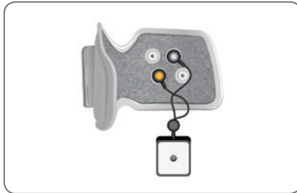
Figure 13-1: Tester Connected to Lower Leg FS Cuff
